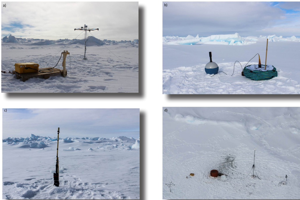
Fig. 3.2.3.2.2: a) Snow depth buoy combined with an IMB (yellow Pelicase), b) SVP buoy, c) marker buoy for outer buoy array, and d) central station with ABiPSO and snow depth buoy
