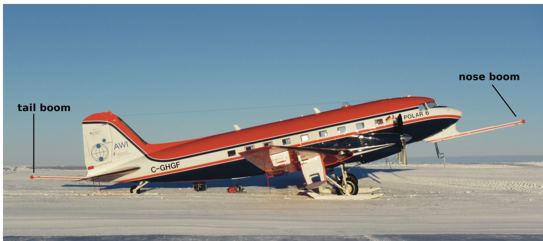
Figure 2.5: Scintrex Cs-3 magnetic total field sensors are mounted in the ends of nose and tail booms on Polar 6 (Basler BT-67 aircraft).
