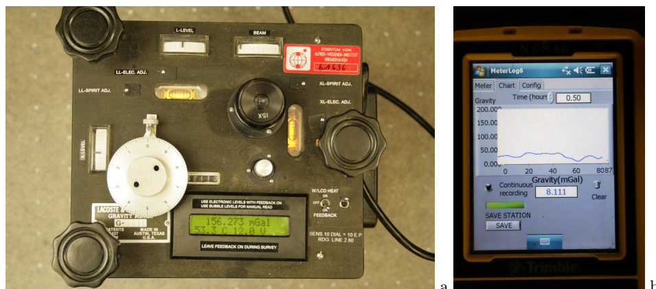
Figure A.1: Feedback system of L&R Meter: (a) LaCoste&Romberg land gravimeter with feedback, (b) handheld computer with feedback control and recording software
