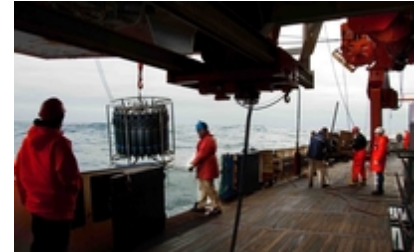
Work on deck: the CTD (left) is recovered, the piston core is being prepared for the next deployment. (photo S. Fietz)
