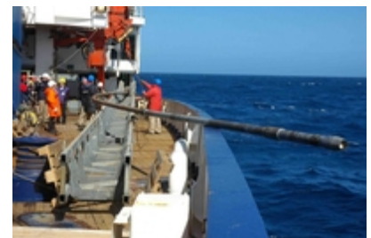
Giant "banana" on deck - the 25 m long piston corer steel tube, bent after penetration in the ocean floor. (photo: Marcel Arevalo)
