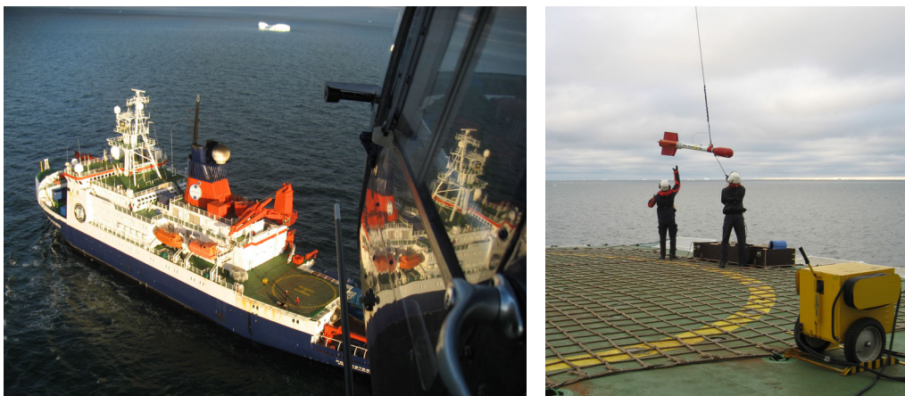
Figure 2.1. Helicopter towed optically pumped cesium-vapor magnetometer operated from R/V Polarstern.
