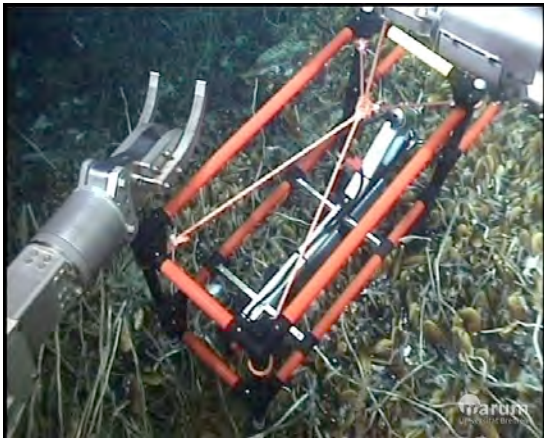
Fig 3. The Eddy correlation system by Frank Wenzhöfer (MPI) to measure integrated oxygen fluxes is placed on the mussel bed.
