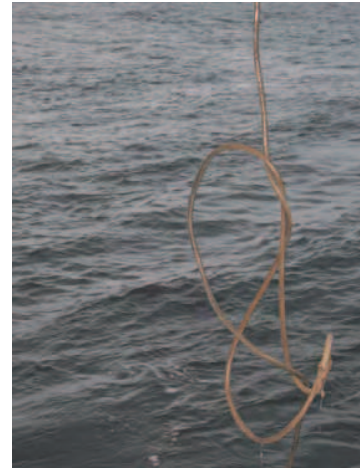
Picture 1: ROV cable “salad” – unfortunately a common view during M76/3b (Source: T Wilkop)
