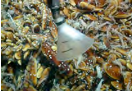
Photo 1: Sampling gas bubbles from a mussel bed ( DIAPIR site; All Photo sources: MARUM)
