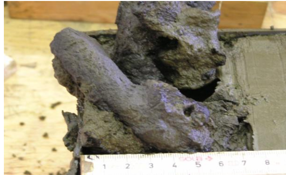
Fig. 4: Large phosphorite concretions sampled with the gravity corer.
