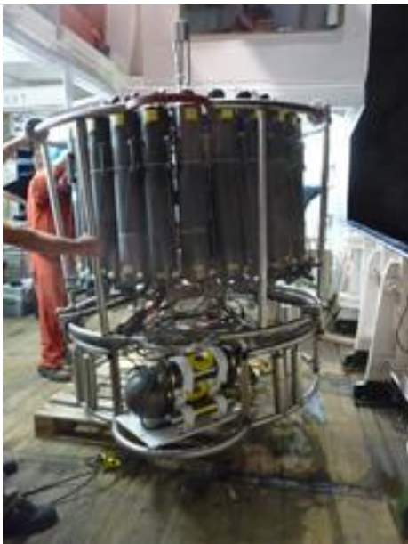
Fig. 5: CTD/rosette instrumented with the in situ mass-spec. TETHYS.
