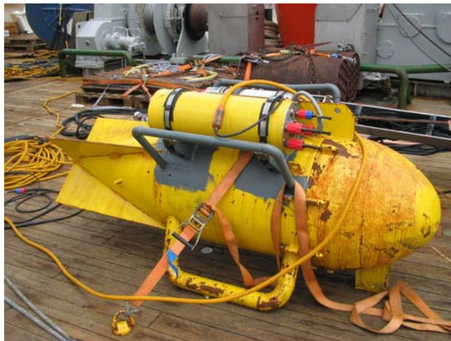
Figure 2: Depressor weight for the deep tow streamer, with attached telemetry (yellow) and positioning cylinders.
