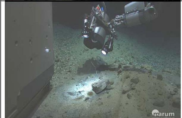
A ROV manipulator arm is shown positioning a large, complex camera system (MegaCam) directly over a rock on the seafloor. The seafloor is dark and silty. The 'marum' logo is visible in the bottom right corner.                                                   | <p>Der ROV Manipulator platziert die MegaCam direkt über dem Objekt der Begierde (Quelle: Marum, Bremen)</p> |
