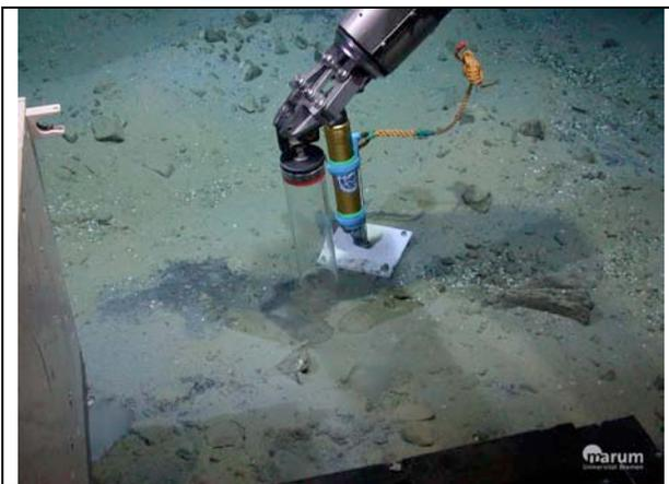
A close-up view of a ROV manipulator arm reaching down to sample the seafloor. The seafloor is covered in dark, silty sediment and small rocks. A small white tag is attached to the end of the manipulator. The 'marum' logo is visible in the bottom right corner. | <p>Beprobung des Meeresboden am Amsterdam Schlammvulkan<br/>(Quelle: Marum, Bremen)</p>                      |
