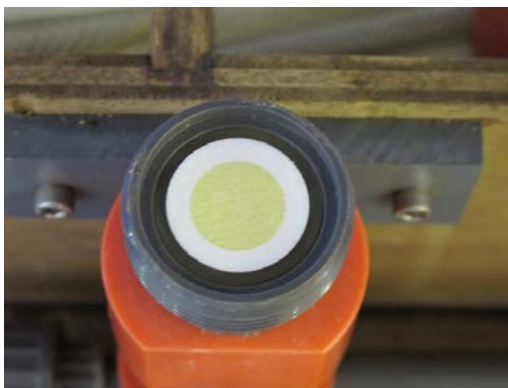
Fig. 4: Green-coloured filter after filtration of several litres of seawater (Photo M. Kaufmann).
