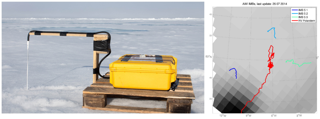
Fig. 9.4: (left) One of the three SAMS type IMB buoys deployed during the cruise. (right) Map of deployment positions and drift tracks of the deployed buoys.
