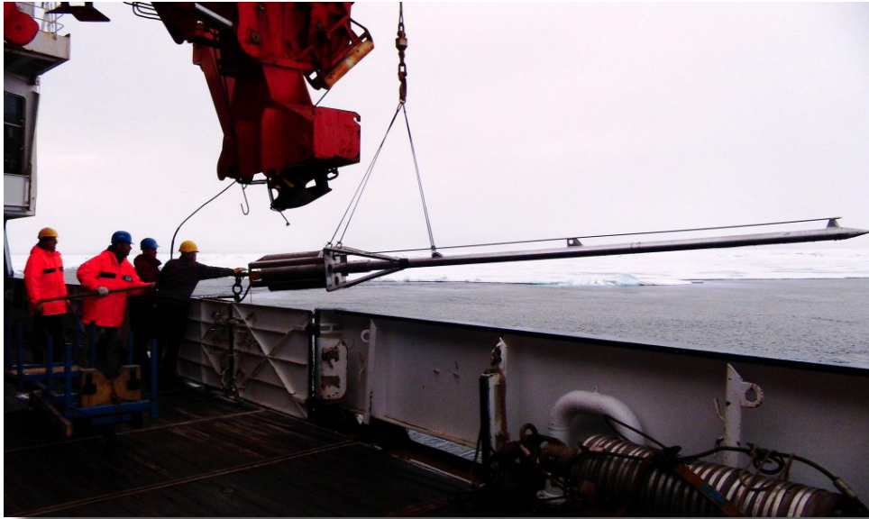
Fig. 5.1: The 6 m Bremen heat flow probe immediately before deployment on Polarstern
