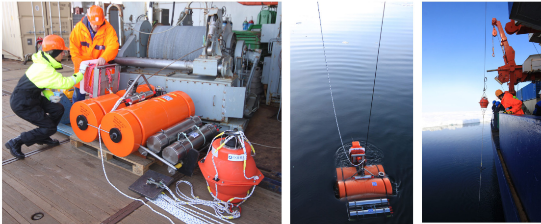
Fig. 4.4: Preparation on deck and deployment of the under ice OBS (images from F. Schmid, AWI)
