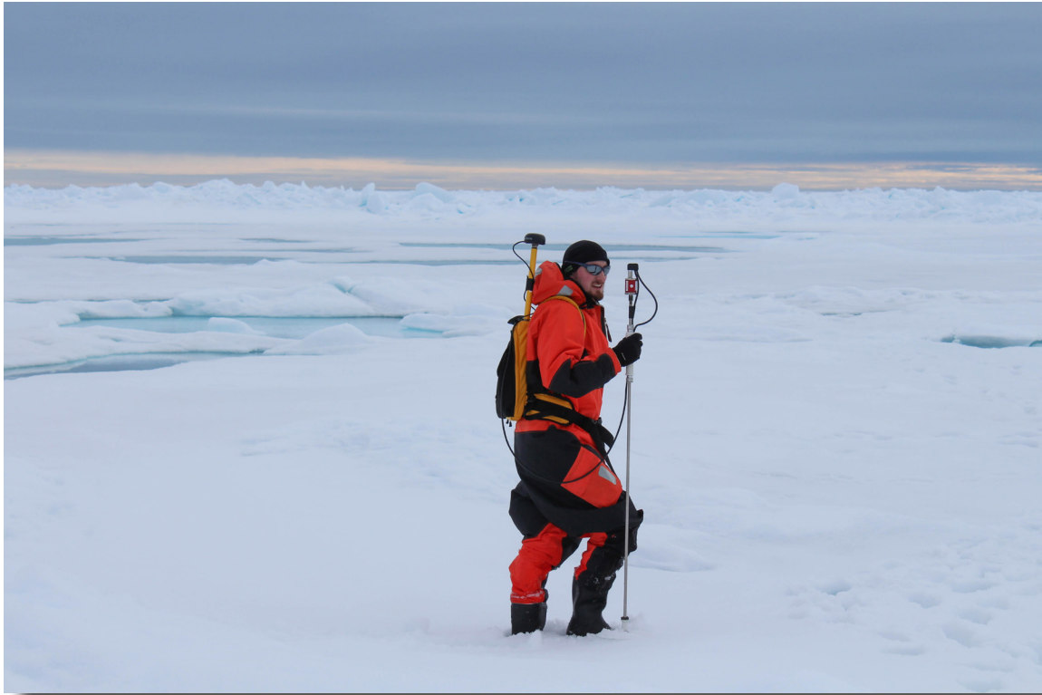
Fig. 9.1: Snow thickness measurements during a helicopter ice-station using the Magna Probe
