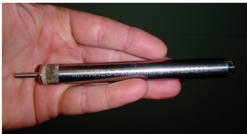
Fig. 5.3: Miniaturized Temperature Logger (MTL), produced by Antares, Stuhr. They operated reliable short term deployments besides some battery issues in cold water ( -0.7^{\circ}\text{C} ) environment. They are rated at 6,000 m water depth, 1 second time resolution and 64,000 samples.
