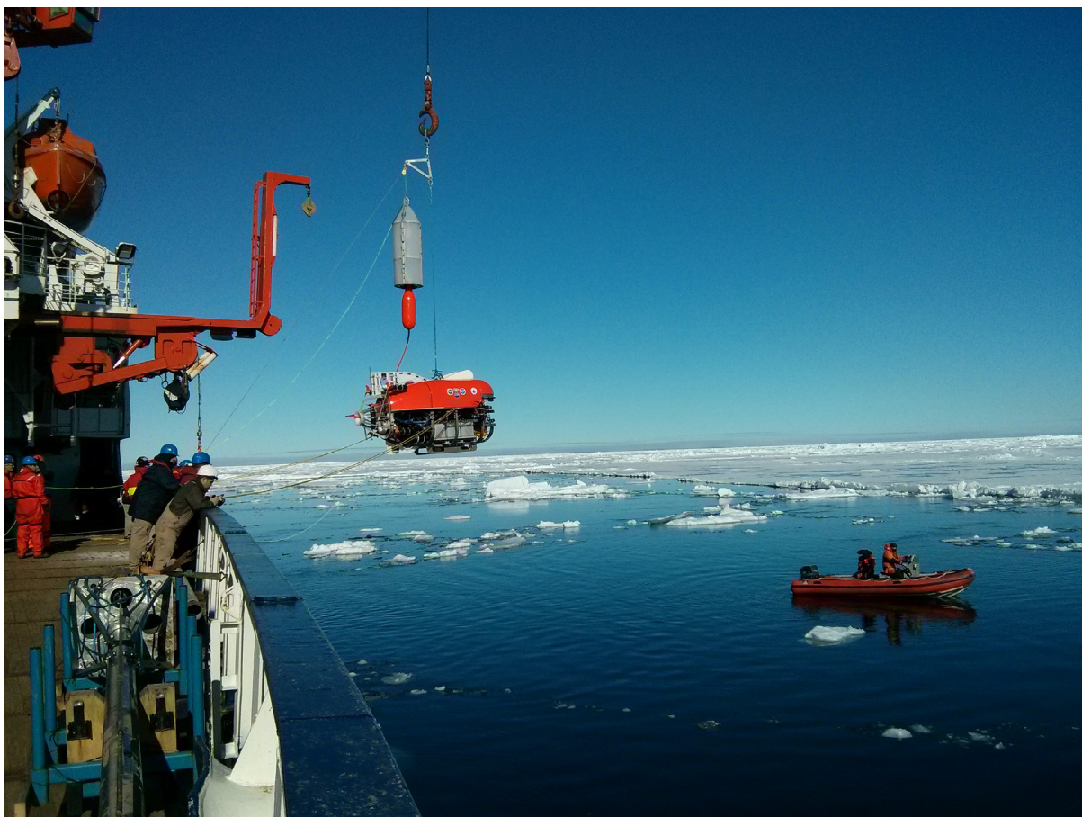
Fig. 10.3: NUI dive 2 launch on July 21, 2014, showing NUI being deployed tethered to the orange tow-body which is mated to the grey depressor during the first part of the launch sequence.
