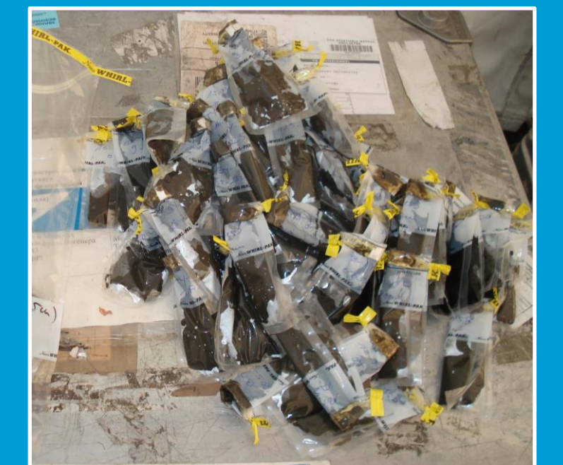
Fig.5: Samples from one core in 0,5 cm slices, cut and stored in Whirlpaks already in the field.
