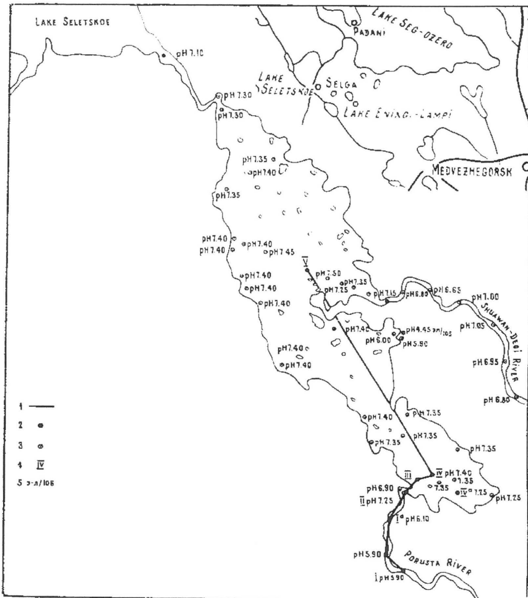
Fig. 2. The schematic map of stations where collected water-samples, measured pH, Eh, the Lake Eningi-Lampi. 1. The line of geochemical section. 2. The stations of water sampling, characterized by chemical analysis. 3. The stations where pH, Eh were measured. 4. Index on geochemical section and on the schematic map. 5. Sample number. Note: the pH values shown on the schematic map for surface water.
