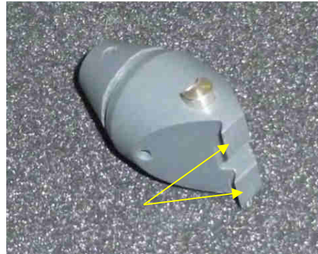
Fig. 8-5a. Locking cone with deflector plates (yellow arrows).
