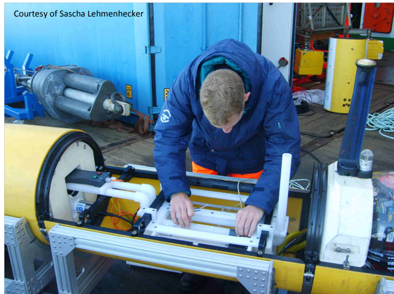
Fig. 4-3. During preparation for the next dive the sample tubes are being inserted.
