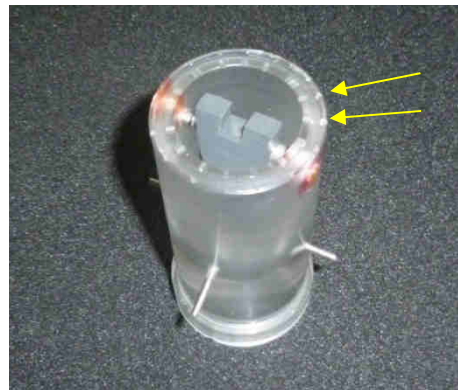
Fig. 8-5b. Acrylic glass model with locking cone inside.
