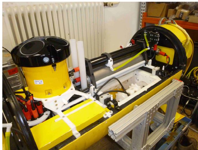
Fig. 11-4. PAUL's payload section with the newly integrated 300 kHz ADCP on the left side of the image. First integration test in April 2015.
