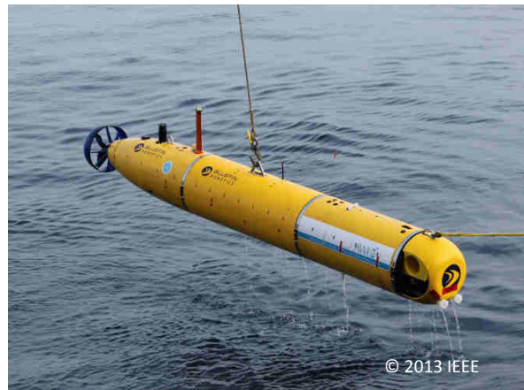
Fig. 5-1. PAUL is being recovered. The float at the nose section is jettisoned.
