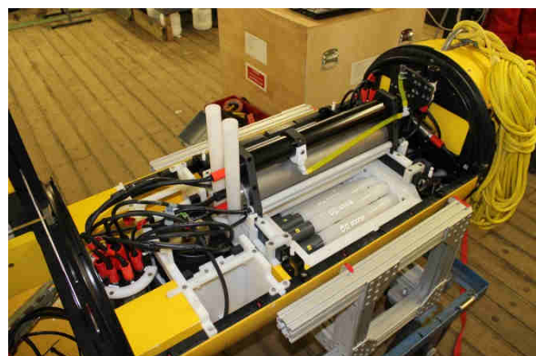
Fig. 1-22. PAUL 's payload section. Note the white tubes which are the containers of the sample collector.
