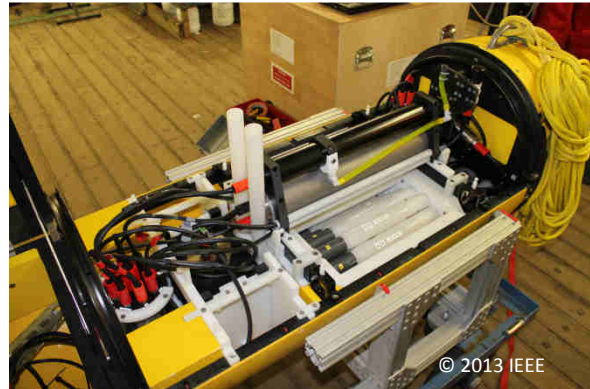
Fig. 5-2. Payload section during ARK 27/2 prior to a dive. The sample containers are already installed.
