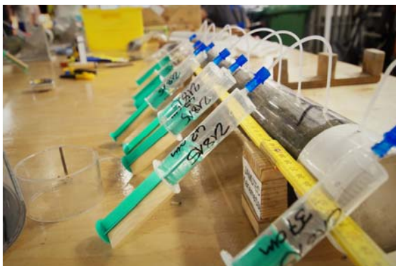
Sampling pore water fluids for geochemical analyses
