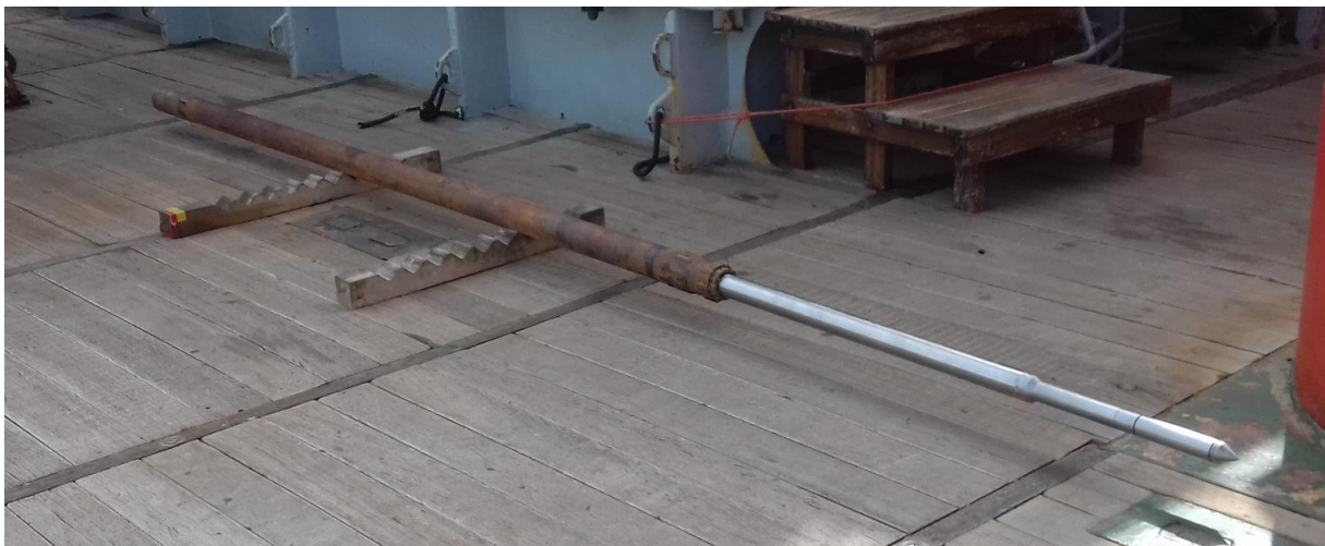
Fig. 1: Configuration of the drill string with the CPT probe.
