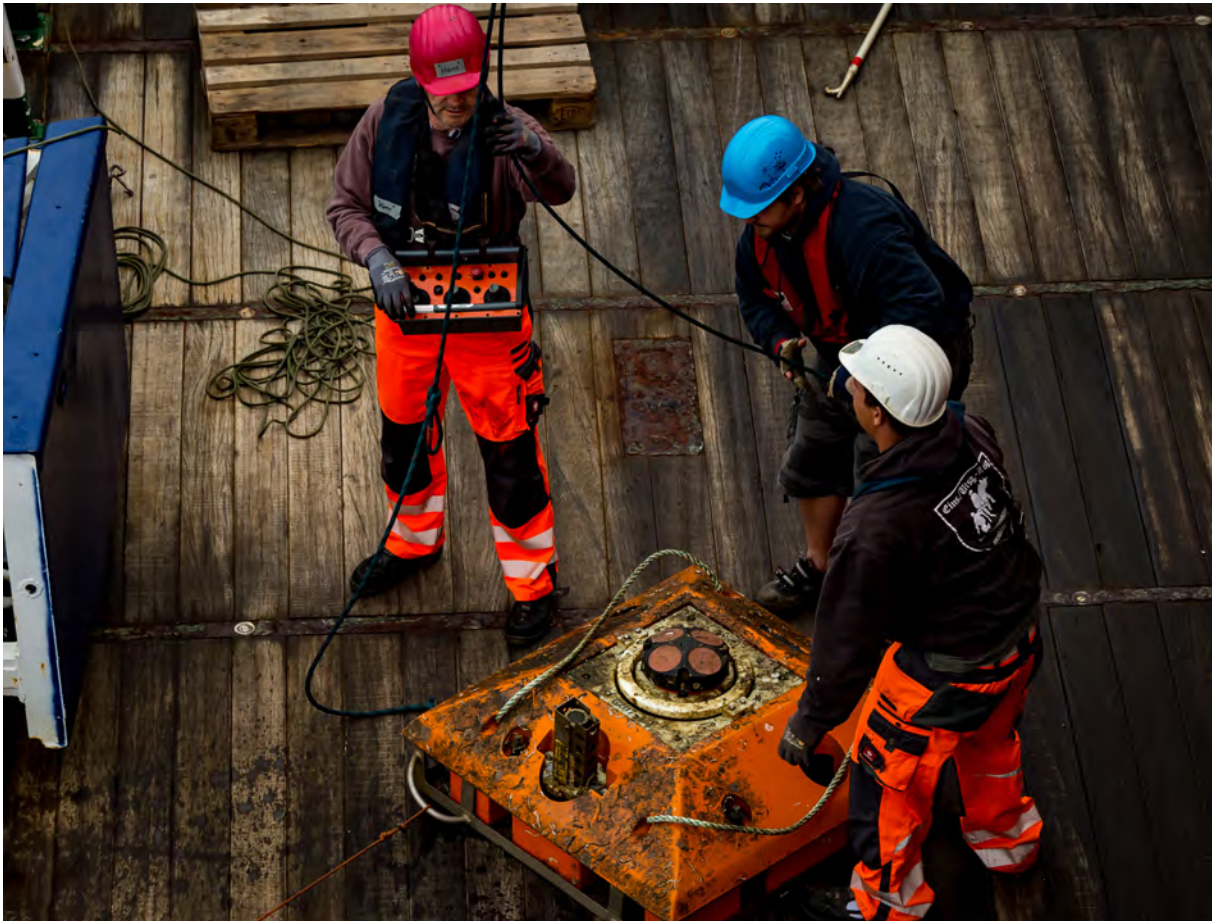
Fig. 2: Successful recovery of the IOW bottom shield equipped with an ADCP on the shelf off Namibia at 18°S (photo: SvN).
