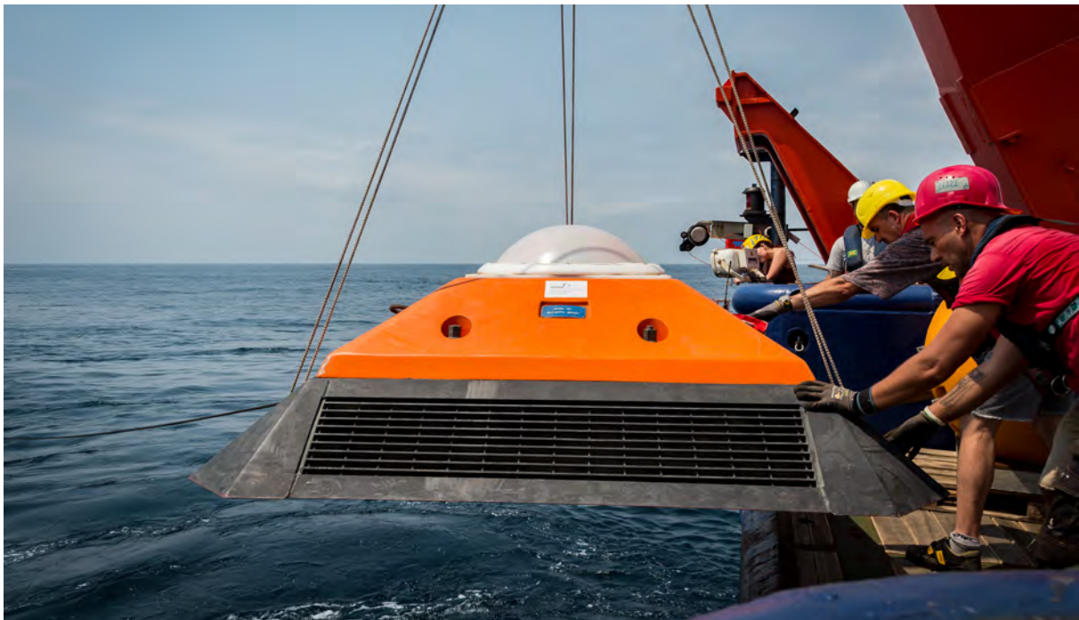
Fig. 2: Deployments of a bottom shield with an acoustic current meter (75kHz Longranger ADCP). The form of the shield is aimed to prevent damage from fishing activities. This time, we added a 1km bottom line that can help during the recovery in case of a damage of the release inside the shield (photo: SvN).
