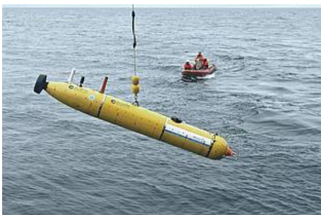
Fig. 2: Deployment of the Autonomous Underwater Vehicle "Paul". (Photo: J. Rapp)
