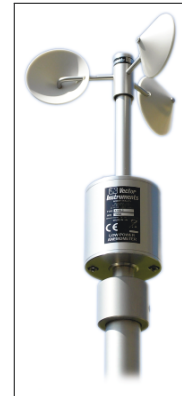
Figure 6: Wind speed sensor
