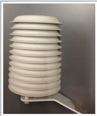
Figure 3: Combined air temperature and humidity sensor
