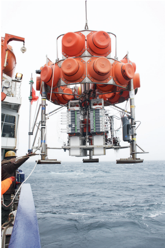
Fig. 11.5.1: Deployment of a benthic lander carrying incubation chambers and a micro-profiling unit
