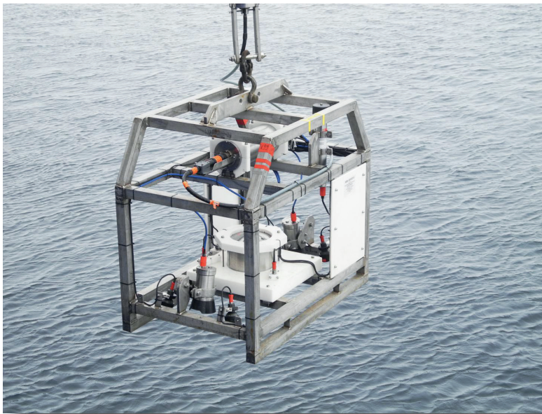
Fig. 11.4.1: The Ocean Floor Observation System (OFOS)
