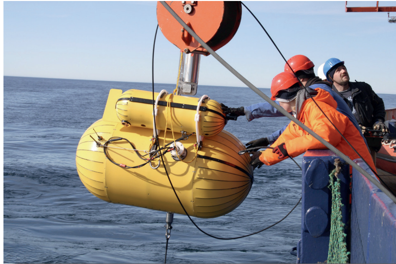
Fig. 11.1.3: Deployment of the SWIPS winch mooring during Polarstern PS99
