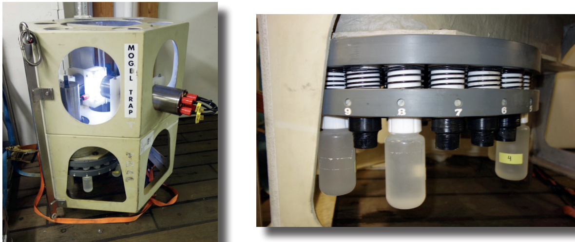
Fig. 13.5: The BOP with the polycarbonate settling column and the camera system switched on (left) and the rotation table with collection cups (right image). The large cups are for long collection periods and the small black cup are filled with viscous gel for short period collection.
