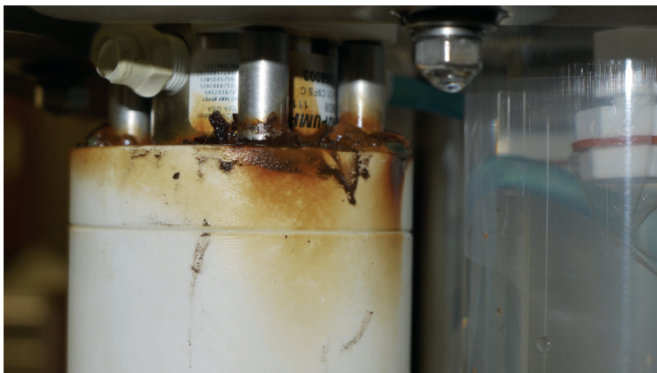
Fig. 11.1.1: Image showing the corrosion on the micro-pump of the McLane Remote Access Sampler RAS-500 deployment at HG-IV, which failed after four sampling events
