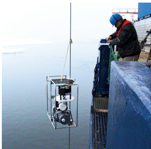
Fig. 15.3: A McLane Large Volume Water Transfer System, or short in-situ pump, that was used for the filtration of large volumes of deep water
