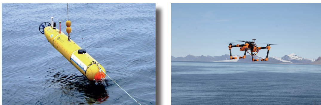
Fig. 7.1: (Left) The AUV is being deployed. Note the orange nose cone, which was attached to mount the microstructure probes. (Right) One of the UAVs returns to Polarstern after a survey flight off the coast of Svalbard.
