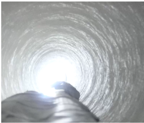
Fig. 4.26: Photo from bedrock section taken with borehole camera in KCC borehole in 2015. Two years after the drilling the unconstrained borehole has started to deform irregularly.
