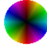
Fig. 4.19: Trend color code: center corresponds to thin section normal, red indicates vertical c -axis orientation.
