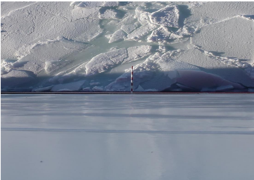
Photograph taken from the starboard side bridge observing deck at 11h30 (GMT) on the 28th of February, during ice breaking. The ice measuring stick can be seen in the centre of the image
