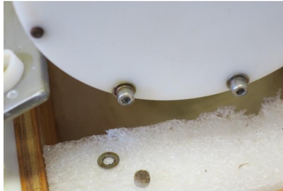
Figure 4.6. 3 : broken screw on Aural#170
