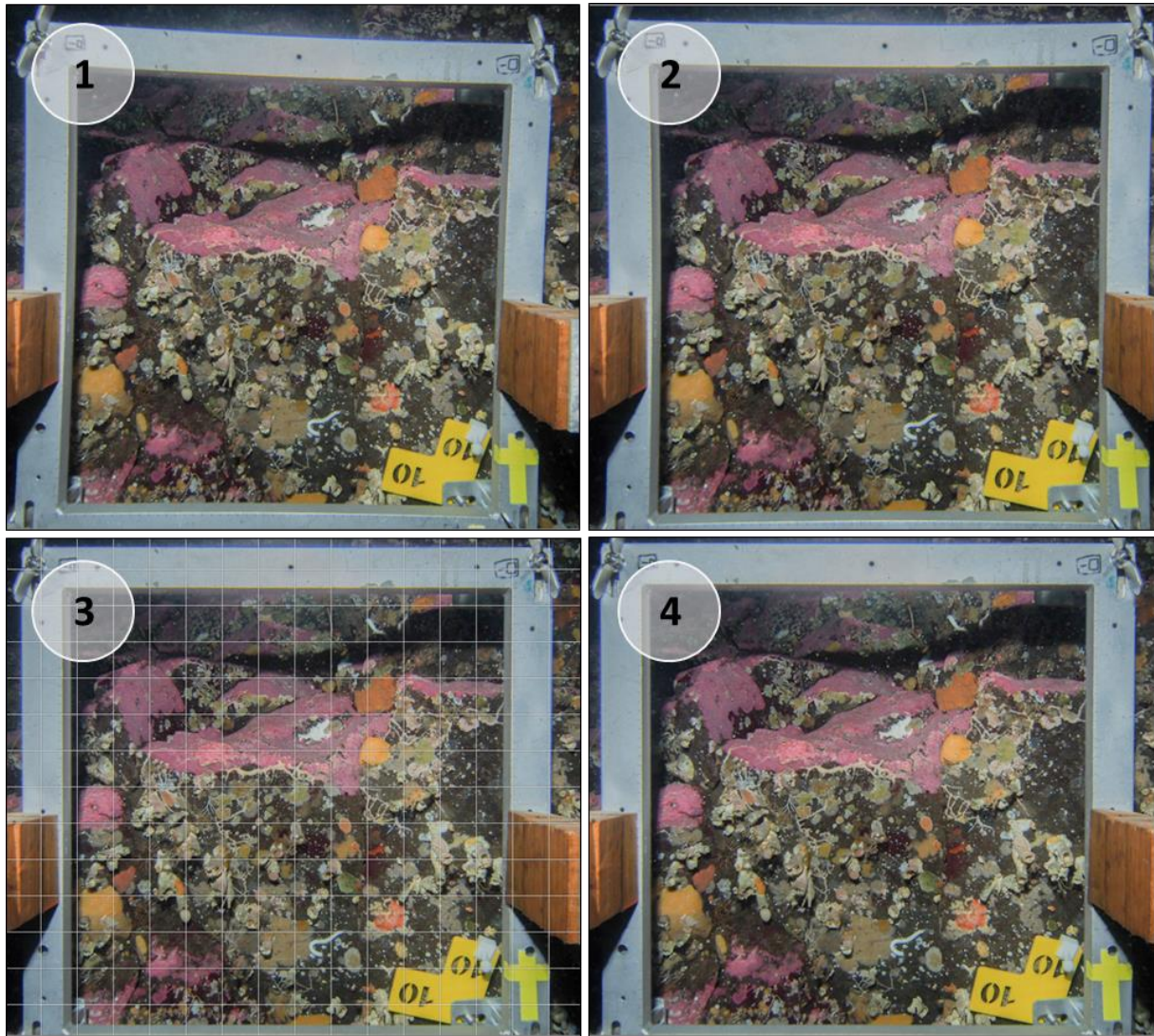
Figure 5: Processing of the raw images prior to analysis: 1) raw image, 2) correction of angle using parallel lines of frame 3) correction of distortion using grid overlay, 4) corrected picture ready for analysis.
