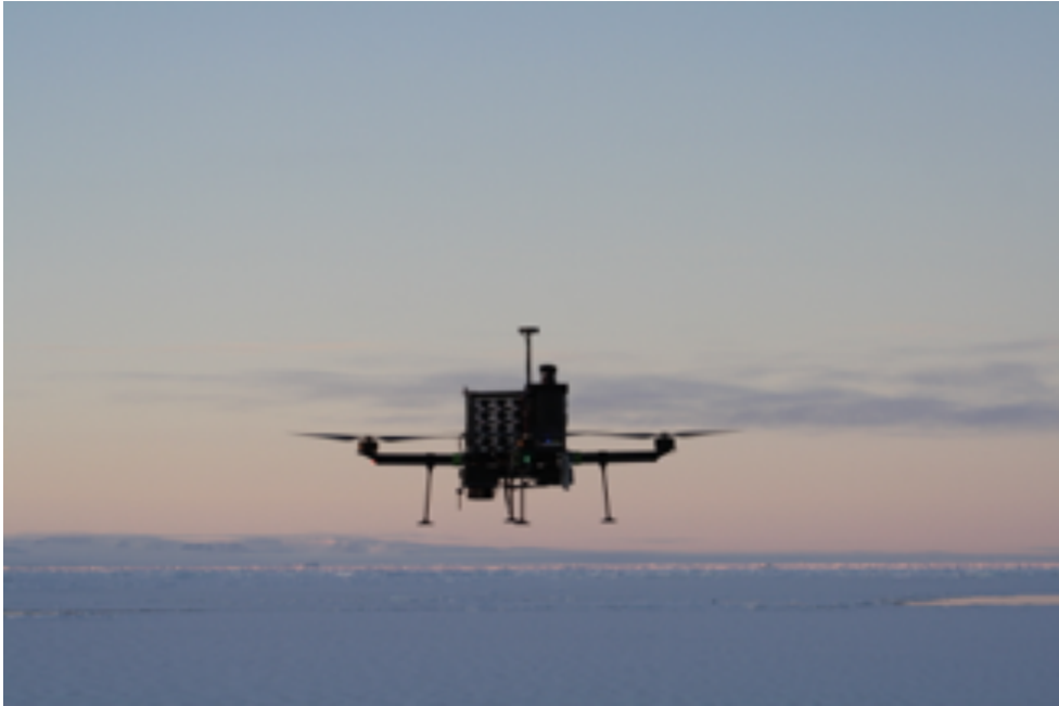
Fig.11.3: Air sampling RPAS in flight
