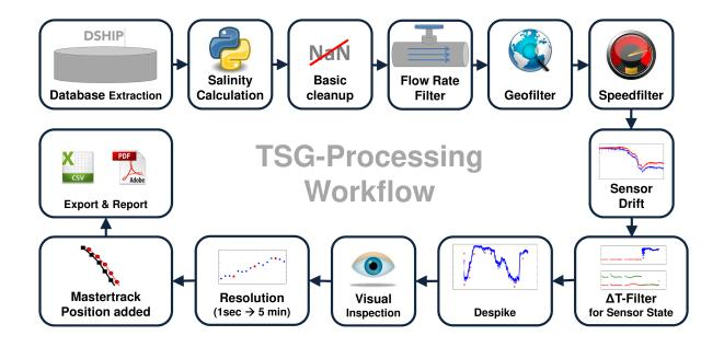
Figure 1: Workflow of TSG data processing
