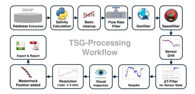
Figure 1: Workflow of TSG data processing
