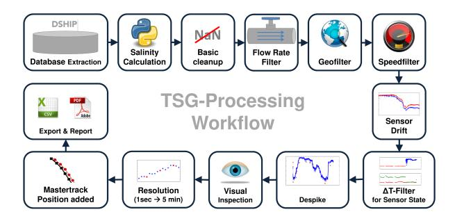
Figure 1: Workflow of TSG data processing
