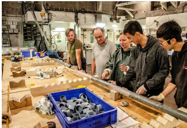
Figure 4: Due to the pressure relief of the sediment cores in the MeBo during ascent in the water column and in the laboratory as well as by gas hydrate decomposition, gas bubbles expand to create voids in the sediment cores. Voids have been taken into account by the scientists when working on the cores (© Paul Wintersteller).
