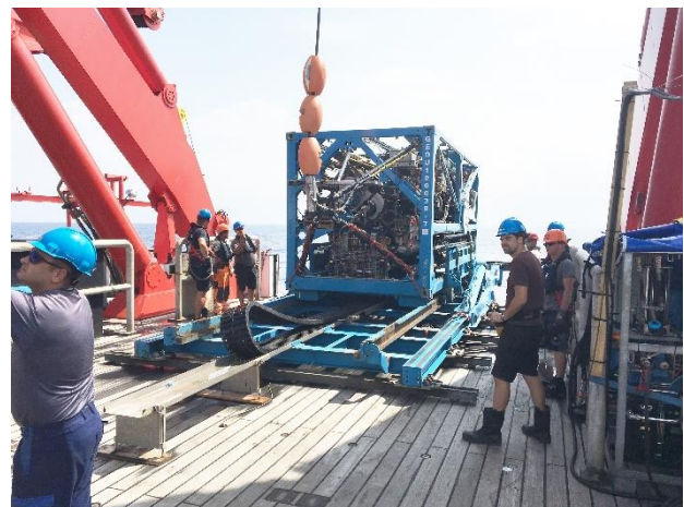
Figure 2: After all the functions of the MeBo200 and its winch have been tested, the drilling rig on its launching system is driven aft over the edge of the ship before being rotated 90 ° to the seabed (© Gerhard Bohrmann).
