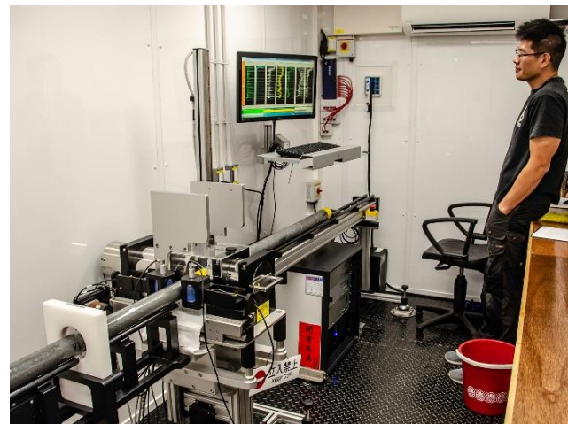
Figure 2: Before the sediment cores are separated lengthwise and sampled, they are examined for their physical properties using the multi-sensor core logger in the container from TORI Institute of Taiwan (© Paul Wintersteller).
