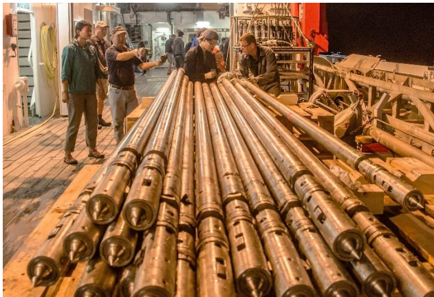
Figure 3: After using MeBo200, the core barrels are removed from the magazines on deck and piled up for the scientists. First, a sediment sample is taken to determine the gases before the sediment-filled liners are pulled out of the core barrels (© Paul Wintersteller).
