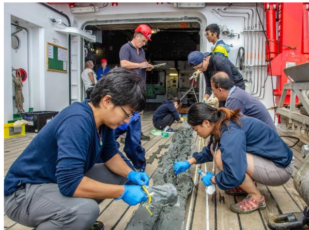
Figure 4: Scientists of the SONNE expedition sampling a core in a bag on the working deck. The use of a tubular bag instead of a plastic liner allows a much faster access to the sediments after the core has been hoisted on board (© Paul Wintersteller).
