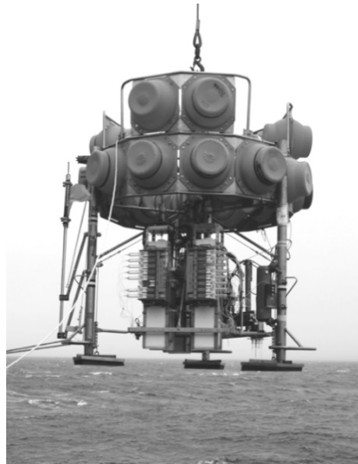
Abb. 10: Bergung eines Freifallgeräts (Bottom-Lander). Fig.10: Recovery of a free-falling system (bottom-lander).
