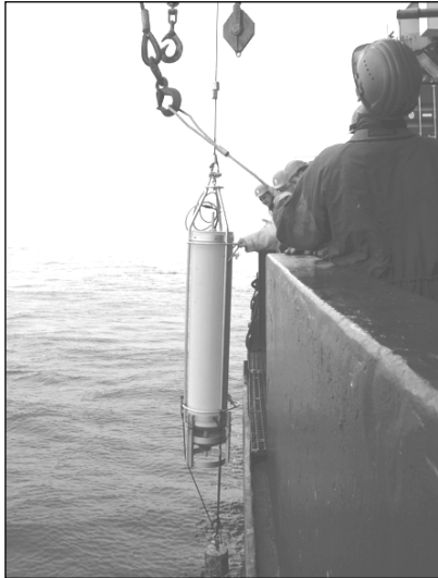
Abb. 9: Einsatz des Marine Snow Catchers. Fig. 9: Deployment of the Marine Snow Catcher.
