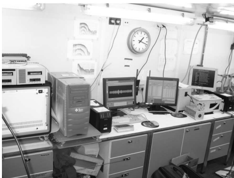
Fig. 11.7 SERCEL SEAL™ digital multichannel seismic system, provided by Exploration Electronics Ltd., and the lab installation of its recordings units.
