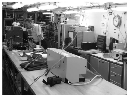
Fig. 11.7 SERCEL SEAL™ digital multichannel seismic system, provided by Exploration Electronics Ltd., and the lab installation of its recordings units.
