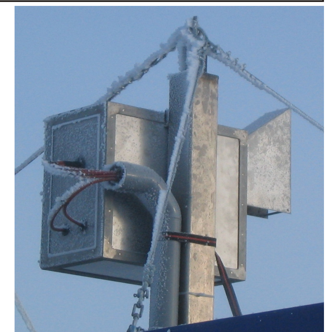
Figure 6: The telescope like it will be mounted on the roof of the container 25m above sea level.
