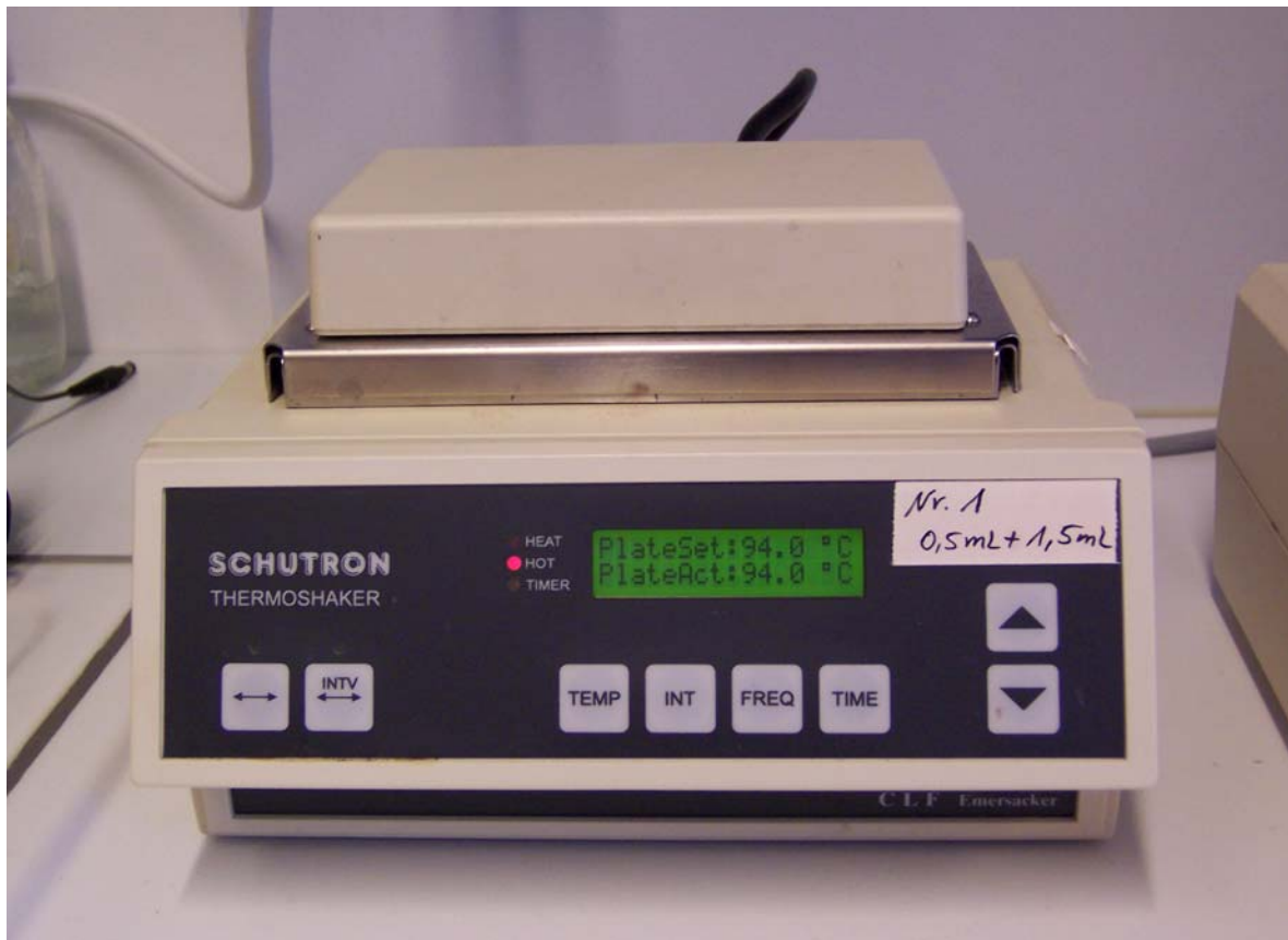
Figure 2. Thermoheater for fragmentation of nucleic acids prior hybridization
