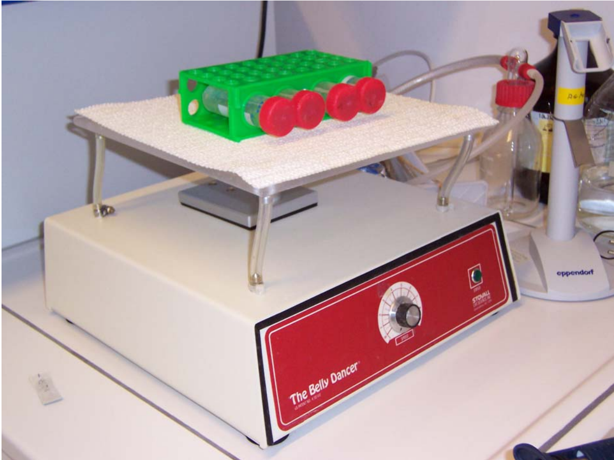
Figure 3. Washing of microarrays by shaking on the bellydancer
