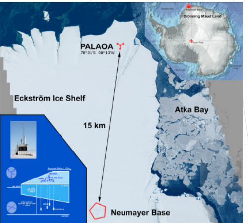
The autonomous recording station consists of an array of up to four hydrophones (300m apart) deployed through the ice shelf (~170m depth). The ice shelf edge is at a distance of 1-3km.
