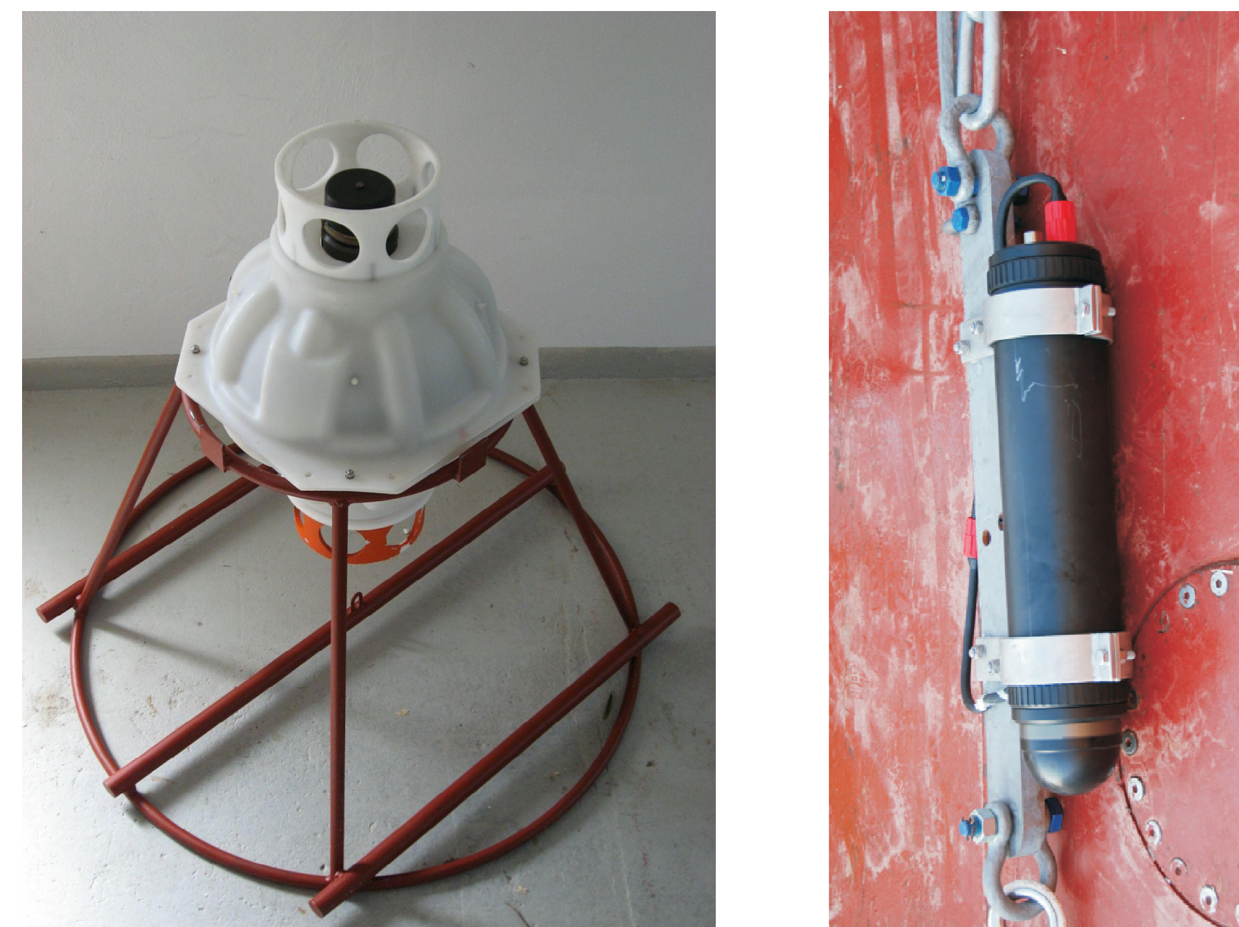
Fig. 2 (left): PACT bottom unit and steel stand. The black cylinder at the top is the HAM-NODE modem; the burn-wire release of the BU is located in the lower cage. For deployment, additional weights are attached between the release and the steel stand.
