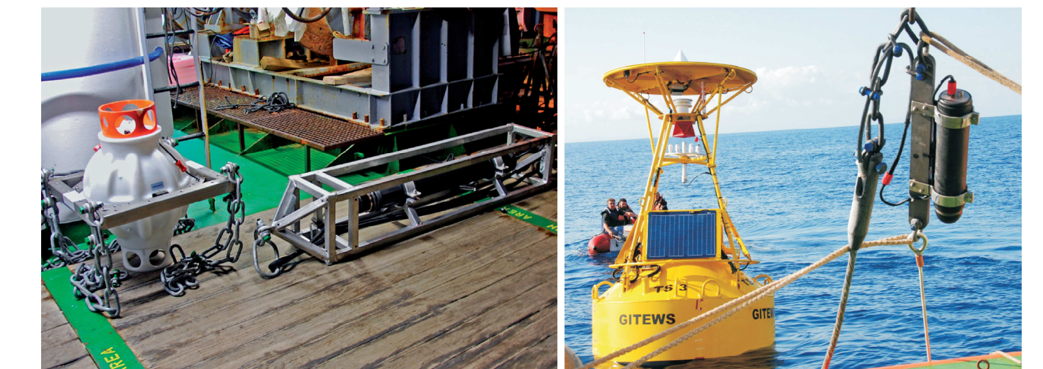
Fig. 6: Left: PACT and HAM.NODE modem prepared for a short-term at-sea test, attached to the ship's hydrographic wire. Right: Test deployment of GITEWS GPS buoy with HAM.NODE modem.
