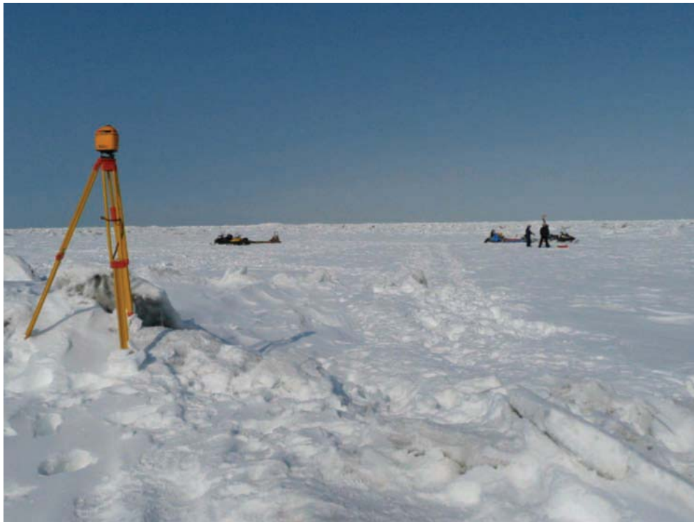
Figure 3.2.11. Rotating laser on a tripod placed on a small ridge. Two people with the laser detector attached to a range pole can be seen in the far back.
