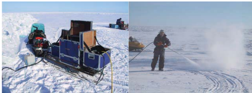
Figure 3.2.6. Operation of hot water drill comprising of a generator, pump, boiler, and hose set up on a sledge (left). A stainless-steel drill rod is used to direct the hot steam under pressure vertically into the ice (right; Photo courtesy Pekka Kosloff).
