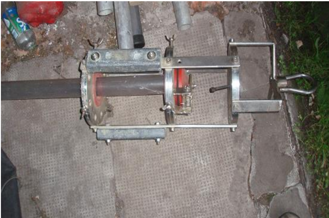
Fig. 6: KB (Kajak - Brinkhurst) core sampler (Model: 603 – 034, Rickly hydrological company, USA).
