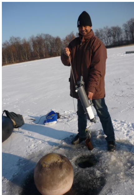
Fig. 5: Water sampler (Ruttner sampler, Hydro-Bios, Germany) used to sample water from 8 m depth of Silver Lake, in this case from the ice in January 2009.
