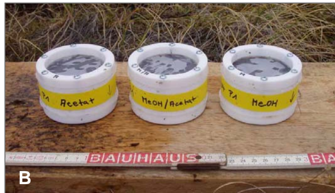
Figure 3-5: Schematic view of the diffusion growth chamber (A) and photograph of the prepared chambers before incubation under natural soil conditions (B).
