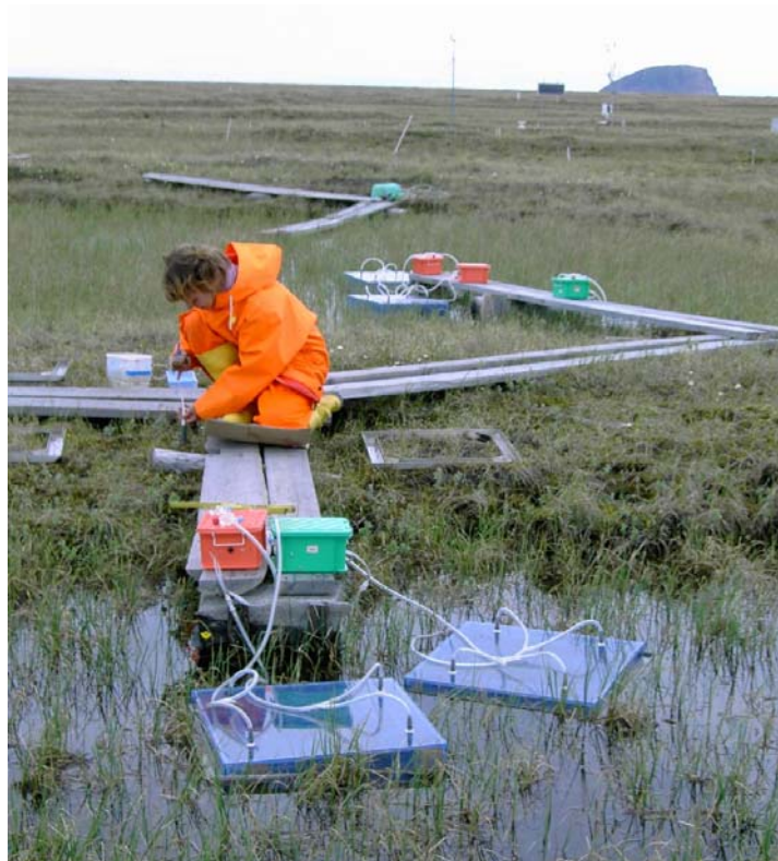
Figure 3-1: Trace gas sampling on the long-term study site on Samoylov Island.
