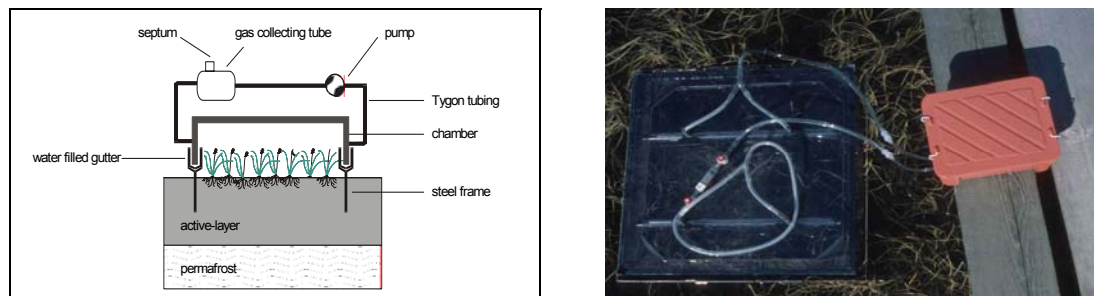
Figure 3-2: Schematic illustration of the methane emission measurement by closed chamber technique (left) and details of the set up during trace gas collection in the field (right).
