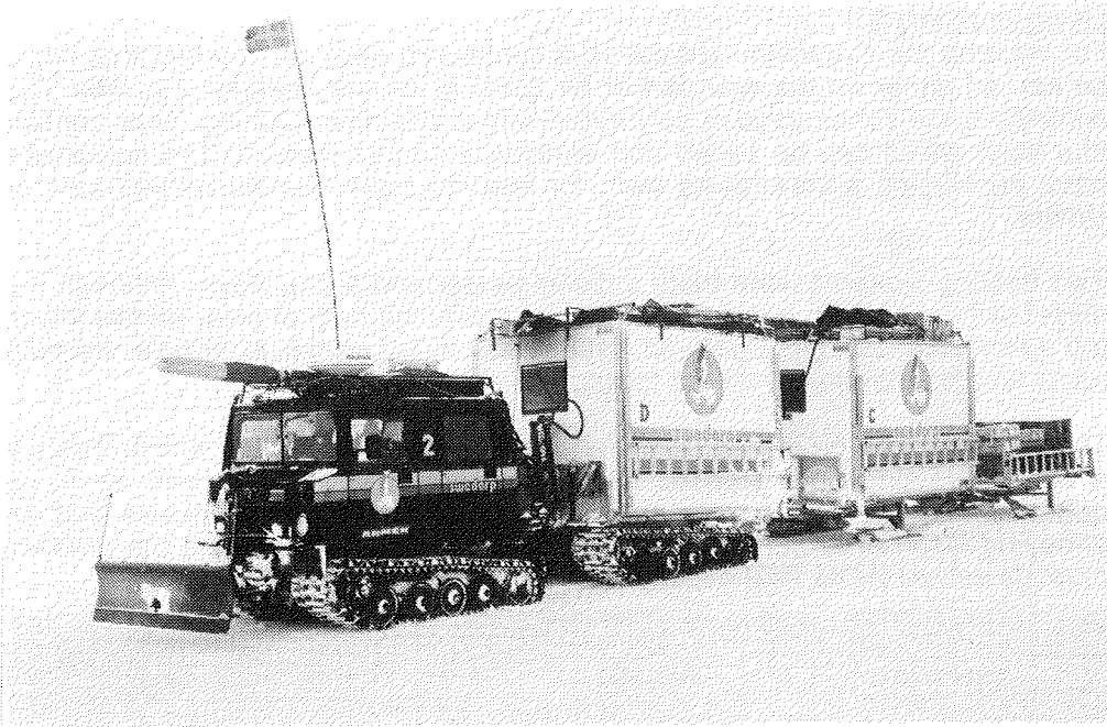
Fig. 38: A train of Hägglund vehicle with a container on its flat-back and two loaded sledges during the traverse to the Heimefrontfjella.
