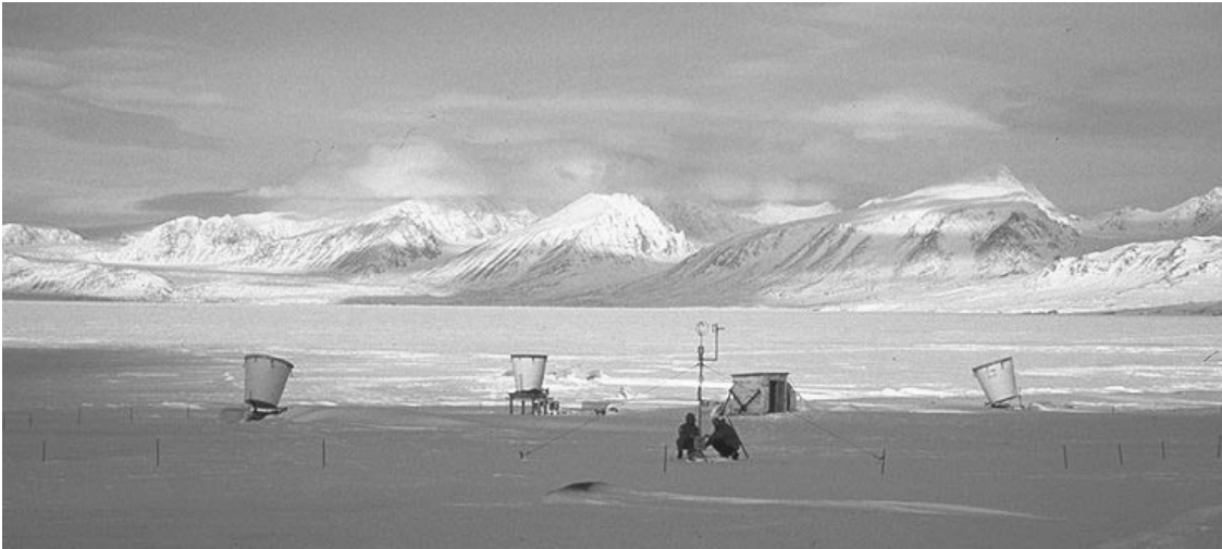
Figure 2.2: Three-axis Sodar, fast-response sensor and radiation station during the field work in Ny-Ålesund.
