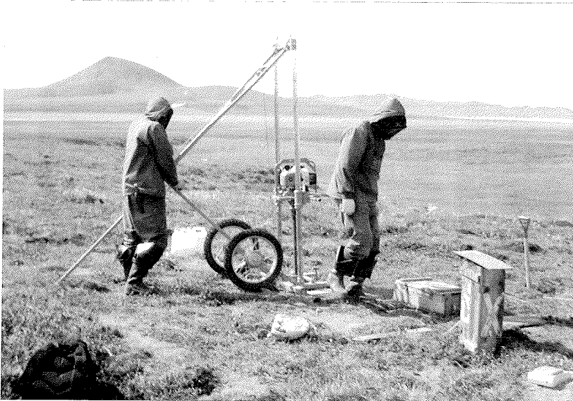
Figure 56: Frozen sediment recovering with the portable shallow coring kit.
