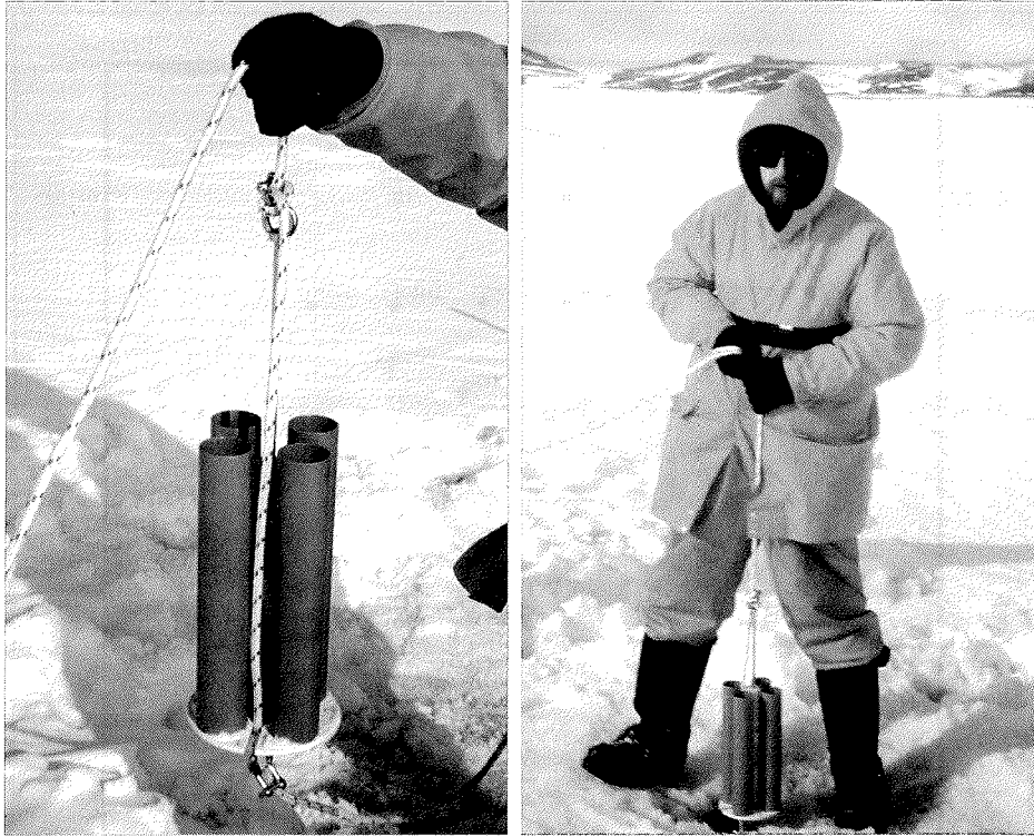
Figure 33: Field work with the sediment traps; Left: detailed view of a trap; Right: deployment during the spring campaign on May 31, 2003.
