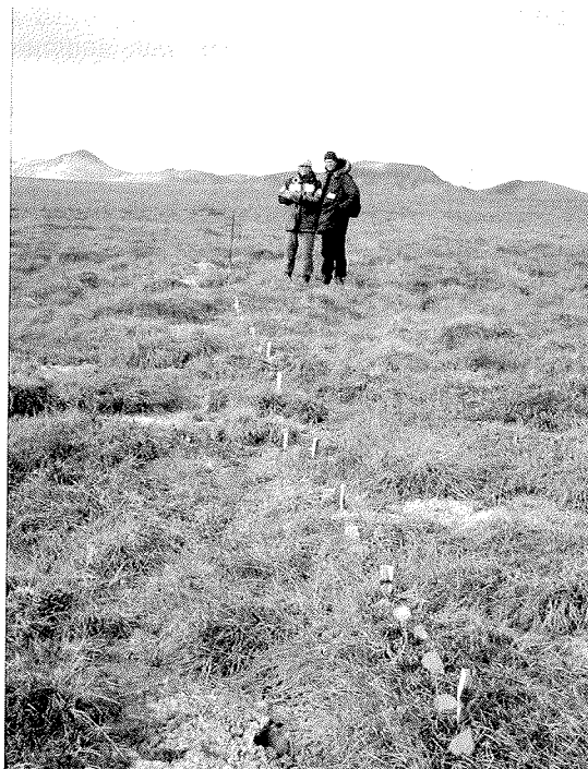
Figure 30: The solifluction monitoring profile in the southeastern sector of the El'gygytyn Crater.
