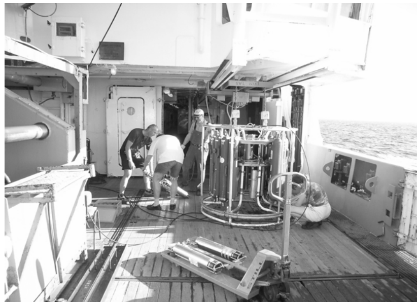
Fig. 2.8: CTD probe with rosette sampler on the working deck of RV Polarstern. In the foreground a dual-release package as used in both re-launched moorings is shown.
