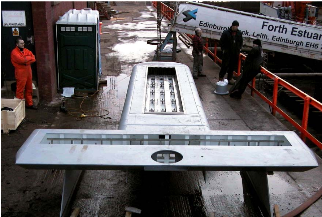
Figure 4 The blister for the EM 120 transducer arrays (2x2 degrees system) designed for “Commander Jack”
