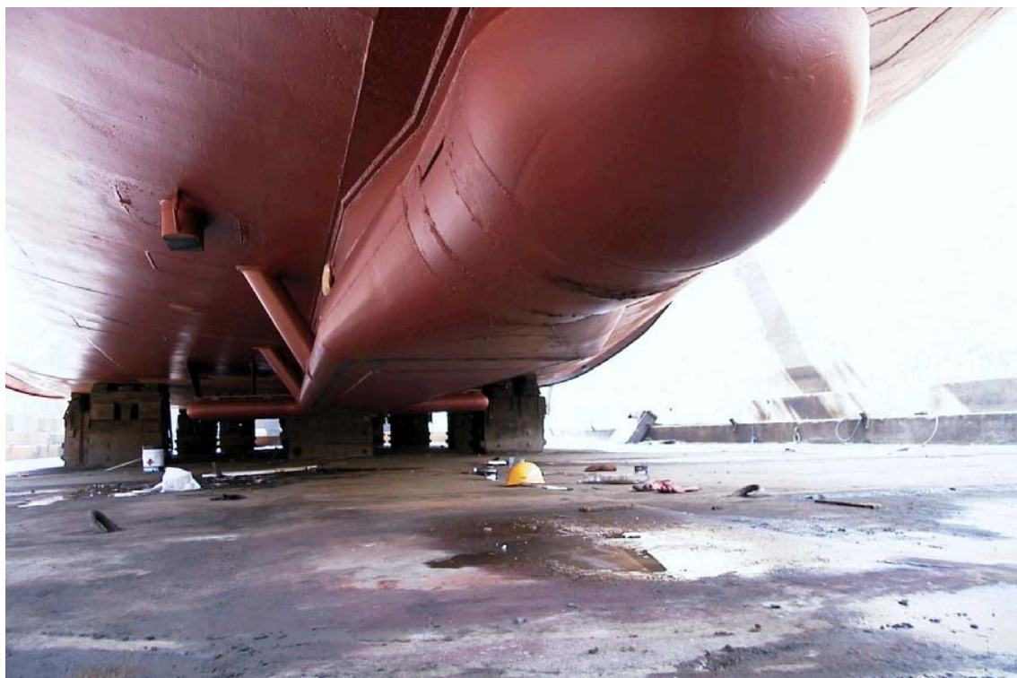
Figure 7 Forward view of the transducer blister on “Bligh”. An EM 1002 transducer array is also mounted.
