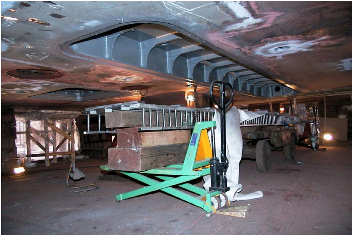
Figure 6 The flush blister for the EM 120 transducer array designed for “James Clark Ross”
