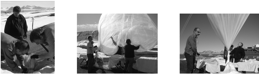
Figure 6.3: Launch preparation of a polyethylene balloon: unpacking(1) and inflating(2 + 3).
