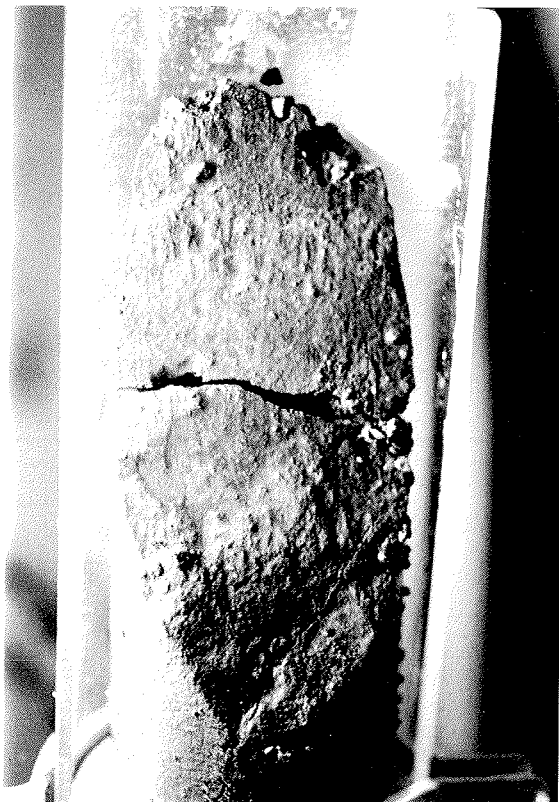
Fig. 4 - Photograph of a high-angle fracture with down-dip striae in the CRP-1 core. Core is 6.1 cm in diameter.
