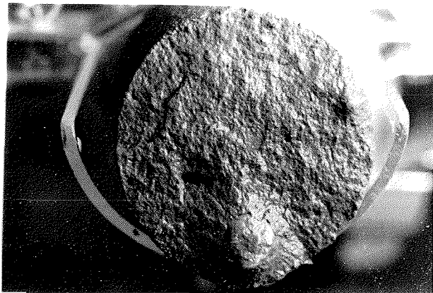
Fig. 8 - Photograph of a subhorizontal fracture with an origin point at a pebble and fine hackle on the fracture surface, demonstrating induced, tensile fracture origin. Core is 6.1 cm in diameter.
