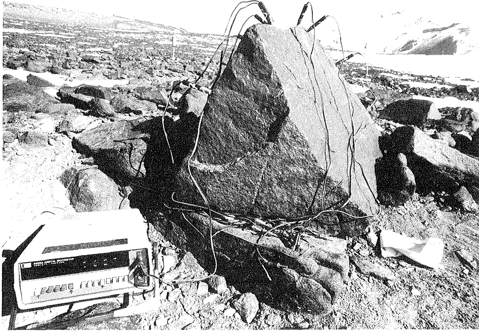
Fig. 6: Rock temperatures under summer radiation vary considerably in the course of a day. Maximum temperatures reach 30° C, but when rock surfaces are shaded the measured values drop fast and dramatically. Thermistors are read at least every 20 minutes around the clock for several days.
