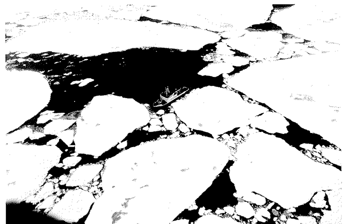
Fig. 2: Picture showing the ice breaking research vessel Polarstern operating in pack ice during the cruise in the Central Arctic in 1991. The ship uses open leads and cracks between the floes to make progress.
