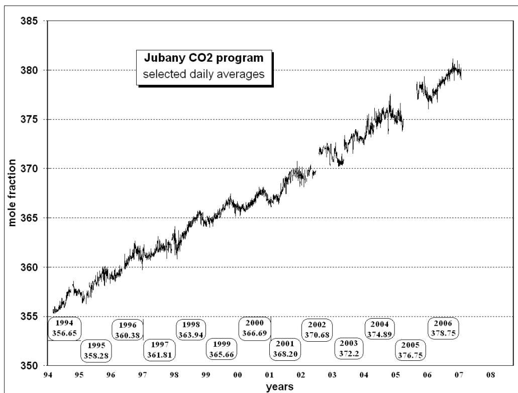
Fig.1: CO 2 daily mean values (mole fraction) selected according to wind and standard dev.
