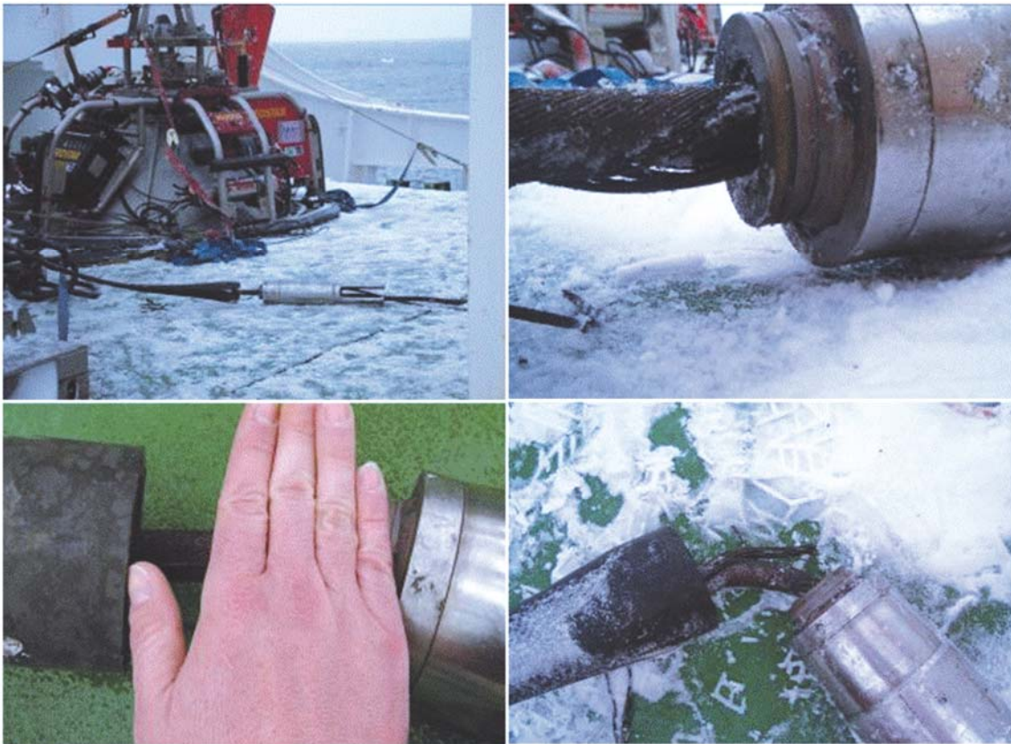
Fig. 15.4: After recovery trial. Details on rupture
