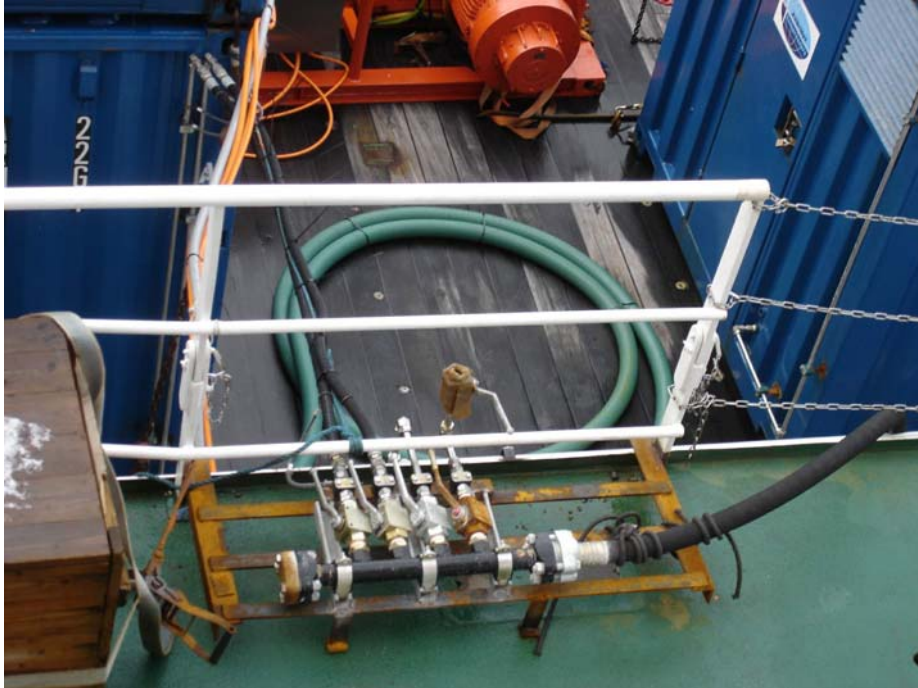
Fig. 10.2. Manifold for high-pressure air supply from compressors to airgun stations.
