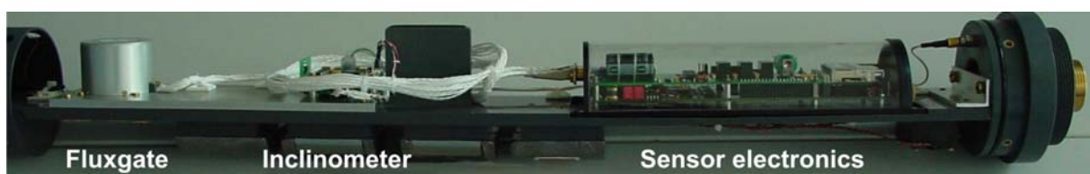
Fig. 9.2: Components inside the fluxgate magnetometer towfish.
