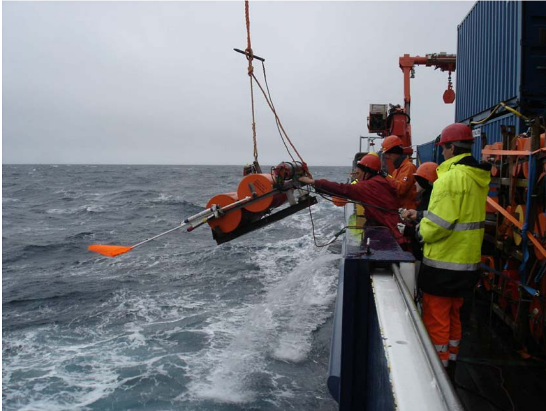
Fig. 10.7. Deployment of OBS system.
