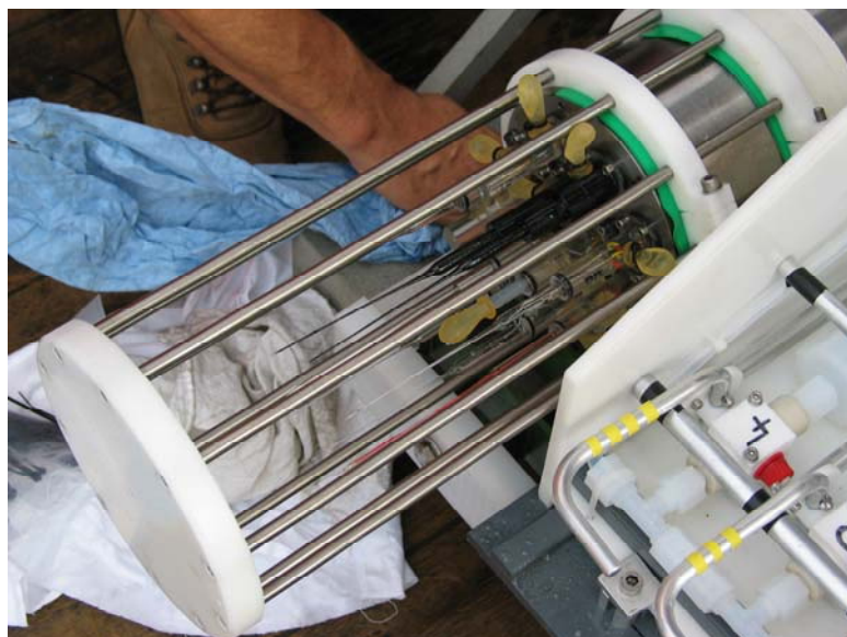
Fig. 3.14 The PROFILUR mounted on the extendable drawer underneath the ROV set up for the dive to come. The microsensors were protected by a cage.
