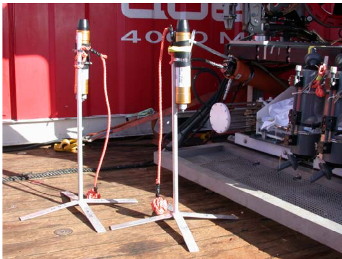
Abb. 3.9 Two homer beacons used for ROV QUEST navigation during M60/3.
