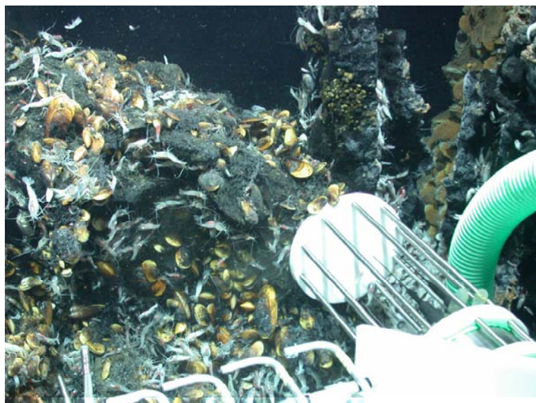
Fig. 3.13 The PROFILUR measuring geochemical data at a Bathymodiolus mussel colony on the active vent structure of IRINA II.
