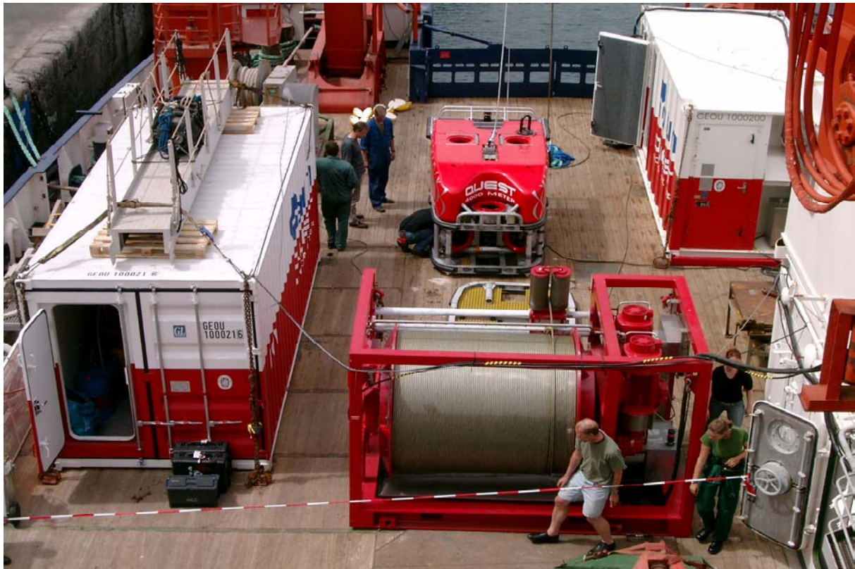
Fig. 3.8: The ROV QUEST system on the afterdeck of R/V METEOR consists of the ROV itself (middle), a control container (right side), a workshop container (left side) and a mobile winch (front).
